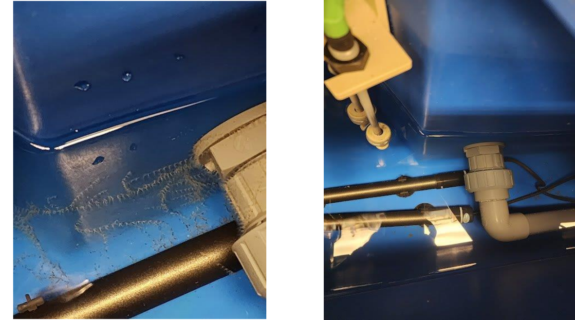
Figure 5-6: A sump before and after cleaning.
